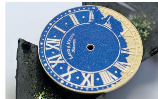
Hand-applied glass crystals fill the relief structure
