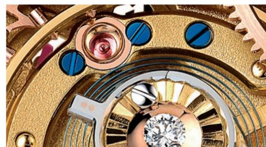
Manually flame-blued screws in the movement
