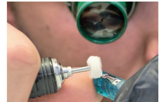
Finissage is applied on a custom-built, domed tool
